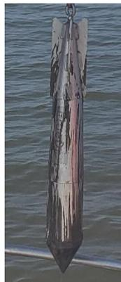
**Fig. 1. *BlueDrop* portable free fall penetrometer after deployment in muddy sediments.**
