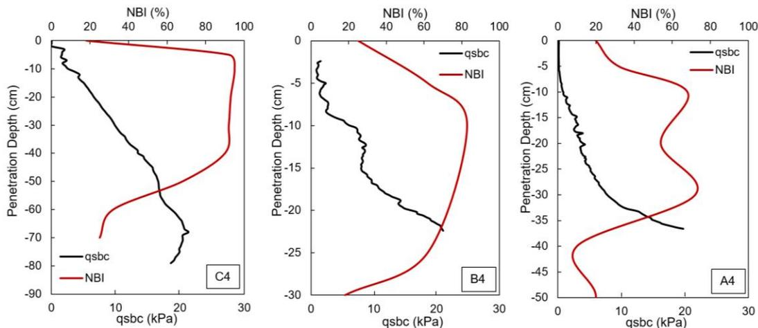
**Fig. 5. Variations in the *q<sub>sbc</sub>* and the *NBI* values with penetration depth at the three sites.**
