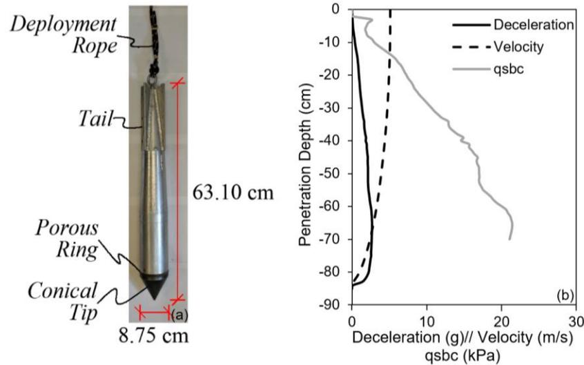
**Fig. 3. (a) PFFP *BlueDrop* and (b) PFFP output deceleration, velocity and estimated  $qsbc$ -depth profiles at C4.**
