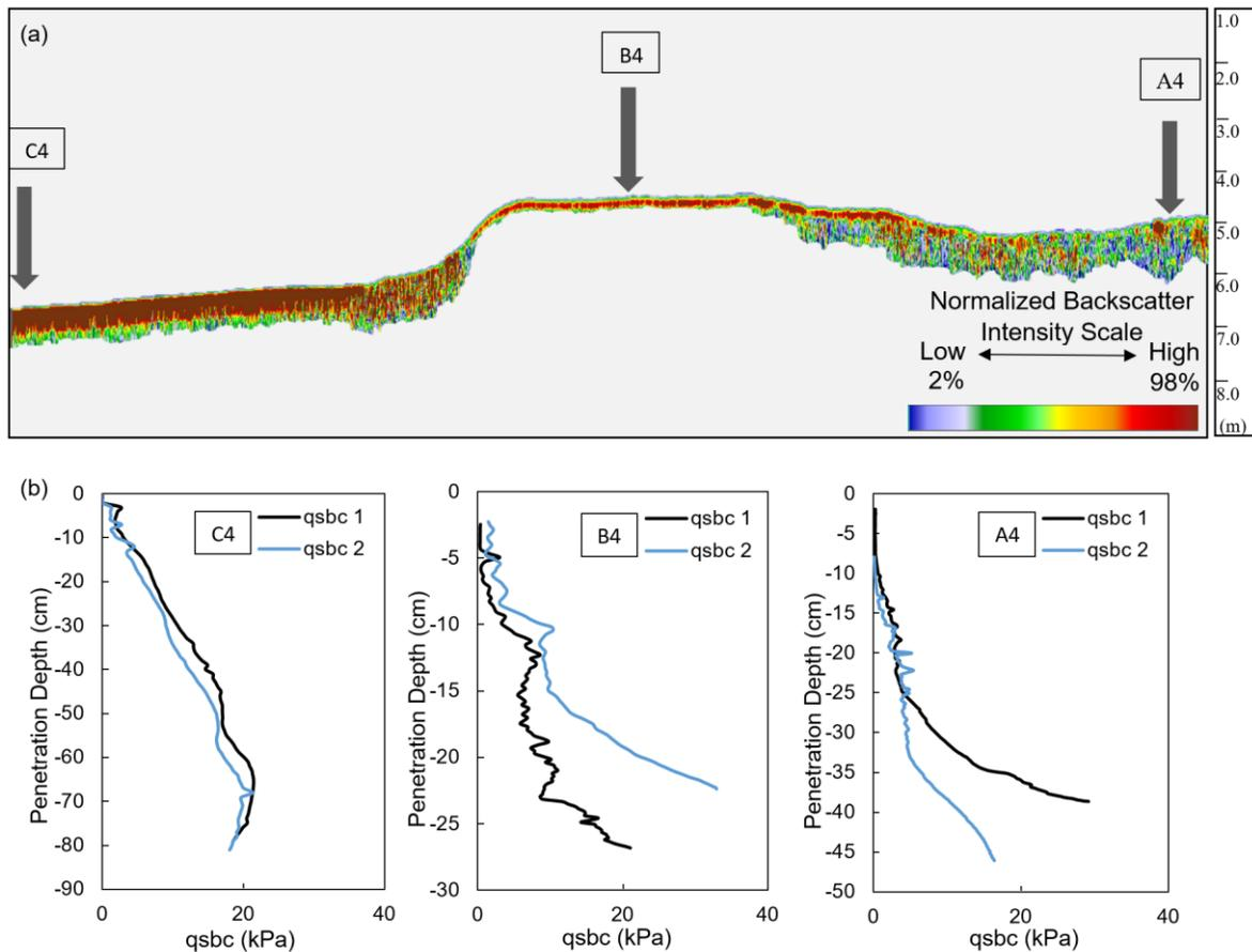
**Fig. 4. (a) Chirp sonar image along transect T4 indicating locations of the three sites analyzed as shown by grey arrows. The color scale refers to different backscatter intensities ranging between blue and red color representing low and high backscatter intensities respectively. The grey color represents water column with depth values shown in the right side bar (y-axis). (b) PFFP deployment results at the three sites.**
